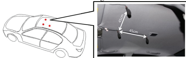
Figure 3. Microphone array setup inside of car
